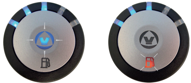
Malfunction in the LPG system
